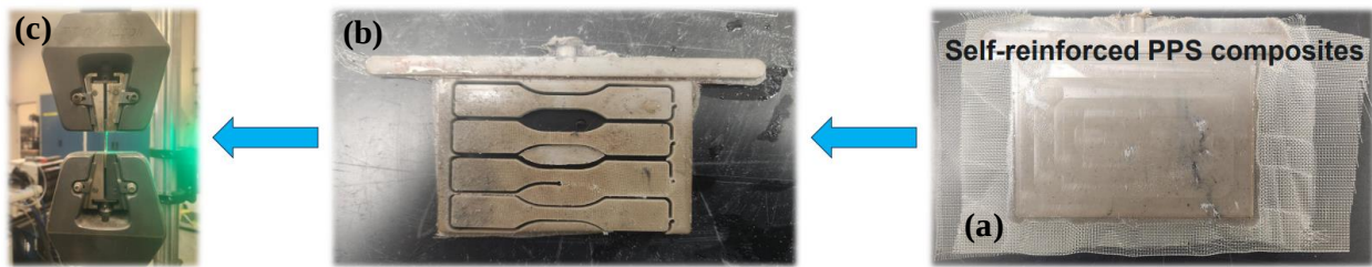
Fig 2. Overview of the process used for cutting the (a) self-reinforced PPS composites using a water jet to produce (b) tensile specimens which were then subjected to (c) tensile testing to gather experimental data.
